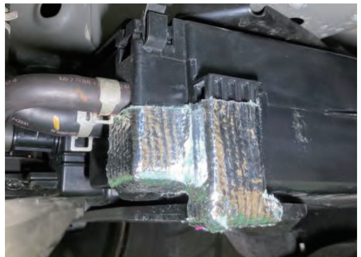
Fig.7 EVAP Canister shape#1 wrapped with the Heat Shield
