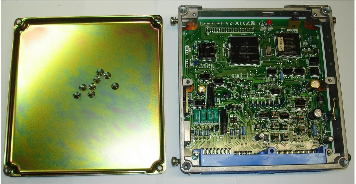
*Tip : The screws that secure the covers will have thread locking compound applied from factory. This stuff really hangs on so make sure you use a driver with a tip which fits the screw head properly. We use a cordless drill. This may seem somewhat excessive but the combination of quality screwdriver tips available and being able to use an adjustable clutch makes for a very effective tool.*
