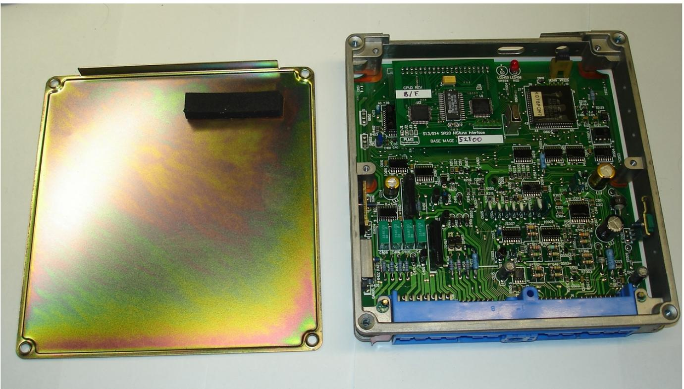
Remove the self adhesive backing from the foam rubber strip and fit it to the lid so that the board will be held firmly in position once the lid is fitted. This is best done by sitting the rubber strip (sticky side up) on top of the Simtek chip which is in the middle of the board, and then carefully fitting the lid.
