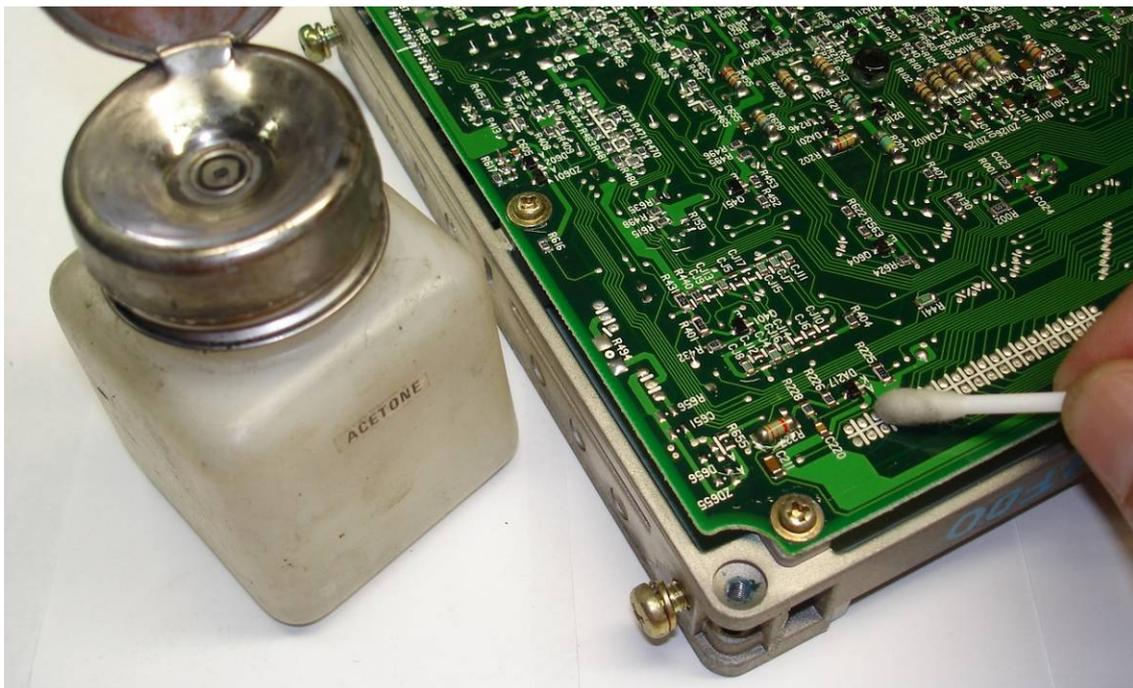
Using solvent or contact cleaner remove the coating around the 20+20 header area on both sides of the board and around the SMD jumpers (see later in document for photos).
