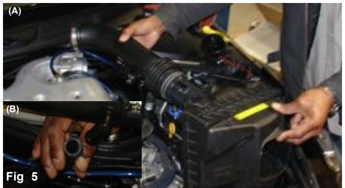
Fig 3 The front air scoop is removed in order to make room for the silicone intake hose.
