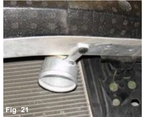
Fig 21 The plastic clip is shown here locating the intake to the bottom of the bumper reinforcement.
