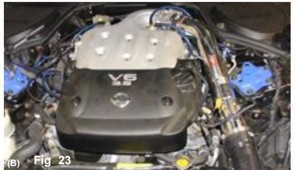
The 3/12" filter is placed over the end of the intake. The clamp on the filter neck is tightened to hold the filter in place (A). Check the entire intake track for best possible fit. Once the intake has been cleared from any rubbing parts continue to tighten all nuts, bolts and clamps. Congratulations, You have just completed the installation of the this cold air intake (B).
